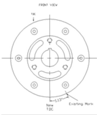
**NEW TIMING MARK PLACEMENT FOR EARLY MG A & MG B APPLICATIONS**
