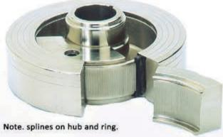
The cutaway above shows internal splines which doubles the contact area, eliminating any possible movement of the outer ring. The outside diameter of the inner hub is splined as is the inner diameter of the outer ring. The elastomer is chemically bonded to the splined areas on Race units. This forms a very positive bond between the elastomer and the steel with double the contact.
